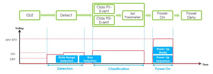
A current problem exists between the detection and start-up phases. Zyxel designs extended commands for user setting:
